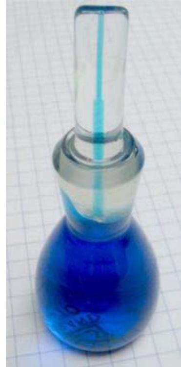
*Pycnometer-empty and full. **NOTE** fluid in stopper*
