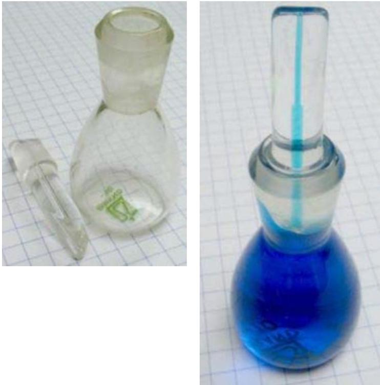
*Pycnometer-empty and full. **NOTE** fluid in stopper*
